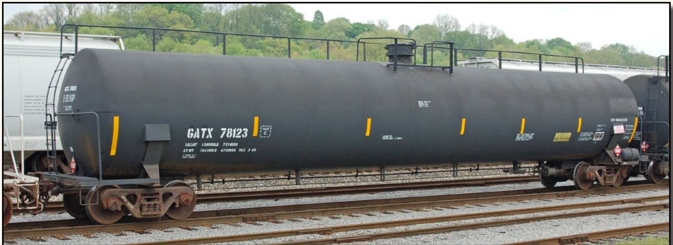
Above: GATX 70551-70585 type T419 were built in September, 1980 as TILX 30001-30035. Below: GATX 78075-78123 type T389 were built in January through March, 1980 as TILX 300200+300364.
