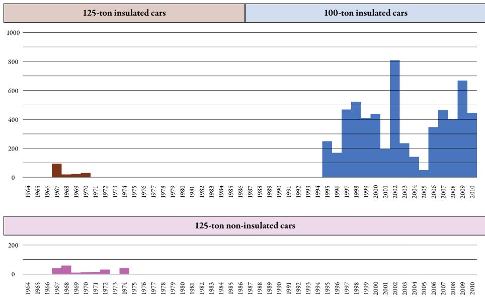
The 100-ton insulated cars are mostly 286,000 pound gross rail load cars used for animal, vegetable or petroleum oils and waxes that would have been carried in 263,000 pound gross rail load T107 cars before 1995. The top six reporting marks in descending order are: ADMX, TILX, MBLX, AZXX, UTLX, and CRGX. Total: over 6,000 cars.
